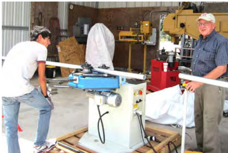
Austin and Gary Kinney cooperate while bending pipe for greenhouse frames.(VBR)
