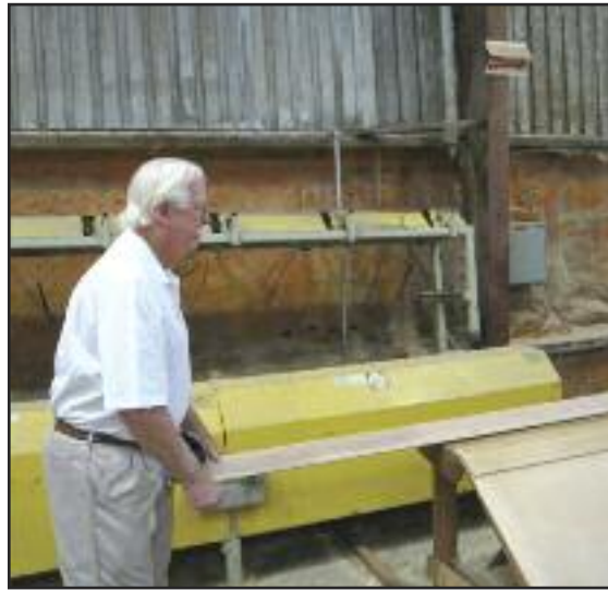
Larry Seal inspects a plank emerging from a planer. (VBR)
